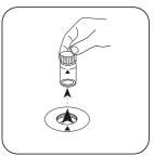
Remove the vial from the sample chamber.
