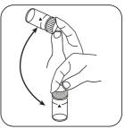
Dissolve tablet(s) by inverting.
