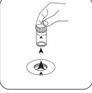
Remove the vial from the sample chamber.
