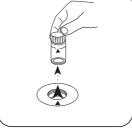
Remove the vial from the sample chamber.
