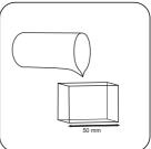
Rinse out vial with prepared **Fill 50 mm vial** with **sample**. sample .
