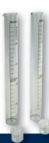
Nessler tubes with immersion tap
