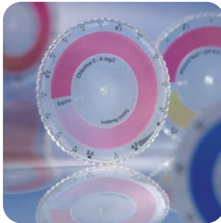
CHECKIT® Discs with continuous and stable scales
