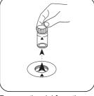
Remove the vial from the sample chamber.
