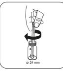
Crush tablet(s) by rotating slightly.
