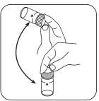
Dissolve tablet(s) by inverting.
