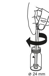
Crush tablet(s) by rotating slightly.
