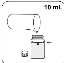
Place **10 mL Nitrite VHR L solution** in the sample cuvette.
