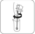
Crush tablet(s) by rotating slightly.
