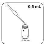
Place **0.5 mL Molyb-denum 2 LR solution** in the sample cuvette.
