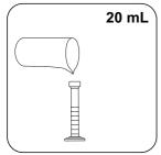
Put **20 mL sample** in 25 mL measuring cylinder.
