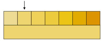
If the hue of the sample is dissimilar to the color standards, making a match visually becomes far more subjective. In the diagram below the nearest color to the sample is shown by the arrow and it is this value that would be predicted by automatic instruments. Visually because of the hue difference the value selected might well be the next standard along to the right. The PFXi instruments would report this sample with an Off Hue factor of 5.
