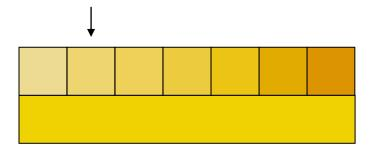
In the following example the nearest colour is still the arrowed standard, but Off Hue factor has been increased to 11. In this example one would expect a visual comparison to give the result as the 6<sup>th</sup> standard along.
