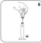
Add 6 drops H<sub>2</sub>O<sub>2</sub>-Reagent Solution.
