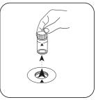
Remove the vial from the sample chamber.
