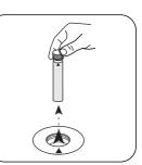
Remove **vial** from the sample chamber.
