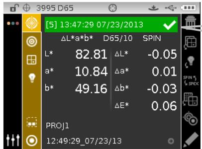
White "check mark" and green bar indicated that the sample passed tolerance.
