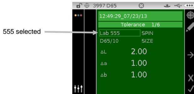
2. Use the navigation control to highlight illum/obs and specular component (SPIN or SPEX) and set as previously explained.
