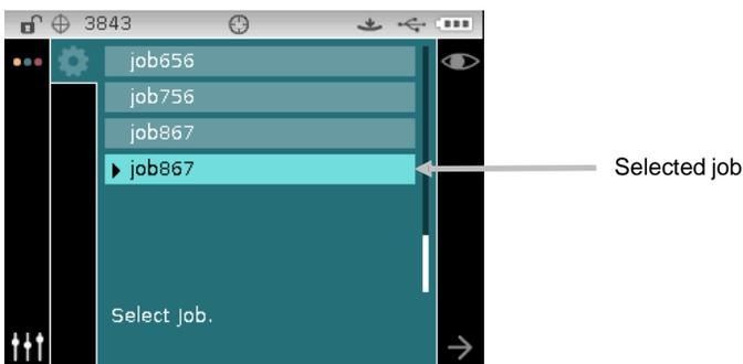
2. Use the **Right** navigation button to move the highlight focus to the Progress column. Use the **Down** navigation button to highlight the Next arrow icon (→) if not selected and tap the **Select** button to open the job. The first step in the job sequence is displayed.
