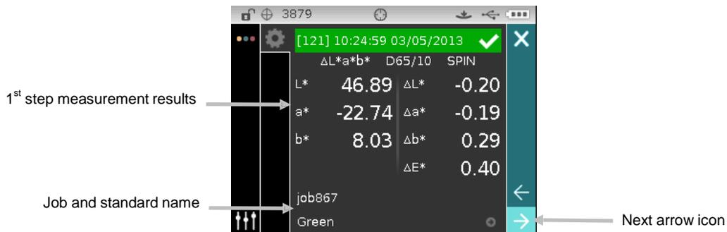
5. Position the instrument on the sample as described on the screen and take the measurement.
