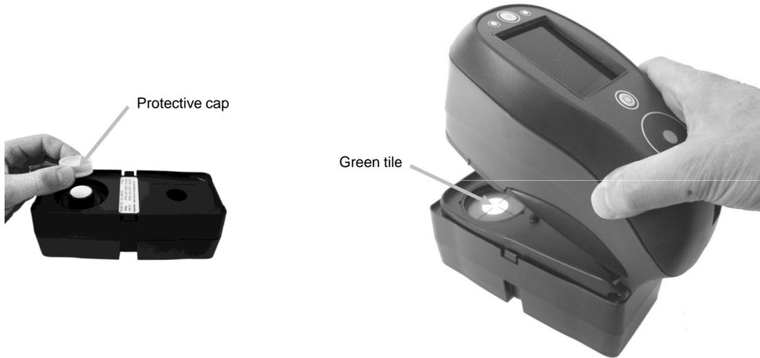
5. Press the instrument firmly to the shoe. Hold steady until the display indicates that reading is complete.
