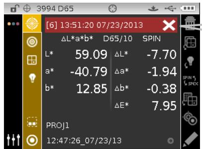
White "X" and red bar indicated that the sample failed tolerance.
