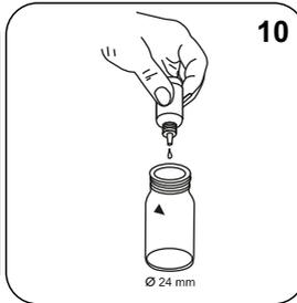
Adicionar **10 gotas Hardness Total Buffer TH2**.
