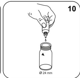
Adicionar **10 gotas Hardness Total Buffer TH2**.
