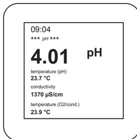
The pH value can be read in operating mode. Stop stirring while doing this.
