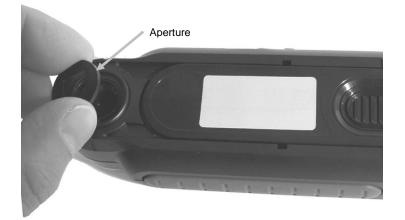
3. Blow short bursts of clean, dry air into the optics port. This should remove any accumulated debris from the optics.
