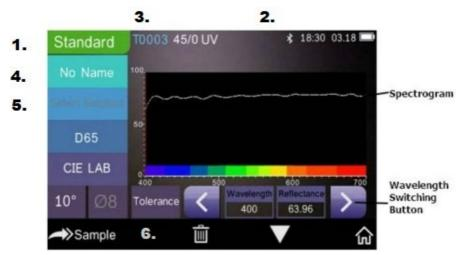
Figure 11 Reflectance of Standard Measurement
