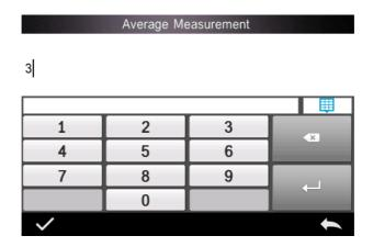
Input a 5 and 5 will be averaged together. The first reading will show 1/5, the second 2/5, the third 3/5 etc. The final average reading will be displayed after the fifth reading.
