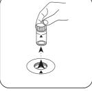
Remove the vial from the sample chamber.
