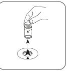
Remove the vial from the sample chamber.
