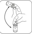
Dissolve tablet(s) by inverting.
