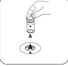
Remove the vial from the sample chamber.
