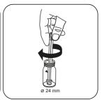
Crush tablet(s) by rotating slightly.
