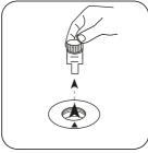
Remove **vial** from the sample chamber.
