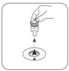
Remove **vial** from the sample chamber.
