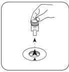
Remove **vial** from the sample chamber.
