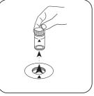
Remove the vial from the sample chamber.
