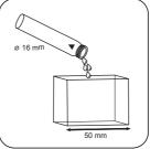
Fill 50 mm vial with prepared sample.
