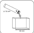
Fill 50 mm vial with prepared sample.
