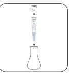
Close the absorption tubes with a plug and fit onto the Erlenmeyer flasks.
