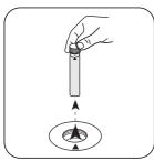
Remove **vial** from the sample chamber.
