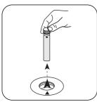
Remove **vial** from the sample chamber.
