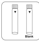
Prepare two reaction vials. Put 2 mL deionised water Put 2 mL sample in the Mark one as a blank.
