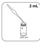
Add exactly 2 mL SPADNS reagent solution top! to the 24 mm vial.
