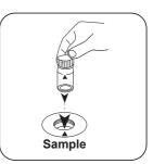
Add exactly 10 mL sample Close vial(s). to the 24 mm vial.
