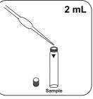
Put 2 mL deionised water Put 2 mL sample in the in the blank.
