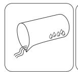
Rinse a beaker with the sample and empty it, leaving a few drops remaining in the beaker.
