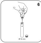
Add 6 drops H<sub>2</sub>O<sub>2</sub>-Reagent Solution.
