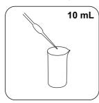
Fill a suitable sample vessel with 10 mL sample F10 powder pack.
