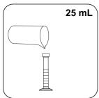
Put **25 mL prepared sample** in 25 mL measuring cylinder.
