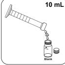
Fill blank with 10 mL prepared sample.
