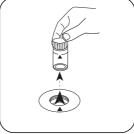
Remove the vial from the sample chamber.
