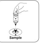
Fill 24 mm vial with **10 mL** Clos **sample**.
