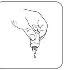
Hold cuvettes vertically and add equal drops by pressing slowly.
