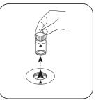
Remove the vial from the sample chamber.
