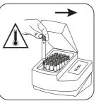
Seal the vials in the preheated thermoreactor for 60 minutes at 100 °C.
