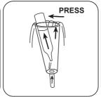
Place a Vacu-vial® ampoule in the sampling vessel. Break off the ampoule tip by applying light pressure against the vessel wall. Wait for the ampoule to fill completely.
