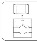
Remove **vial** from the sample chamber.
