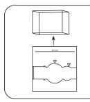
Remove **vial** from the sample chamber.
