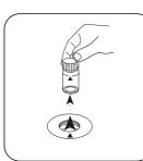
Remove the vial from the sample chamber.
