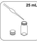
Fill one of the digestion vials with 25 mL of prepared sample.
