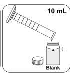
Fill blank with **10 mL** prepared, not digested sample.
