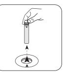
Remove vial from the sample chamber.
