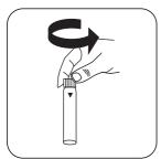
Open a digestion vial PO<sub>4</sub>-P Acid Reagent.
