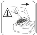
Remove the vial from the thermoreactor. (Note: vial will be hot!)
