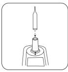
Place the ampoule in the sample chamber.
