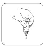
Add Hardness Calcium Buffer CH2 drop by drop to the same sample until colouration turns from light pink to red. (Note: make sure to swirl the vial after adding each drop!)
