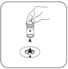
Remove the vial from the sample chamber.
