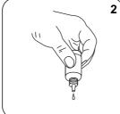
Add 2 drops Acidity / Add Hardness Calcium Alkalinity P Indicator PA1. Buffer CH2 drop by drop
