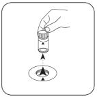
Remove the vial from the sample chamber.
