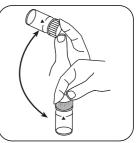
Dissolve tablet(s) by inverting.
