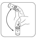
Dissolve tablet(s) by inverting.
