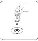
Remove the vial from the sample chamber.
