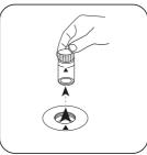
Remove the vial from the sample chamber.
