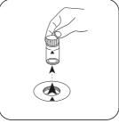
Remove the vial from the sample chamber.
